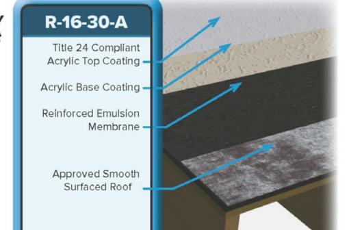
WeatherWeid R-16-30-A is a completely seamless roof system designed for installation over nearly all smooth and granule surfaced roof systems\*. \*Contact WeatherWeld for more information on acceptable roof types.
