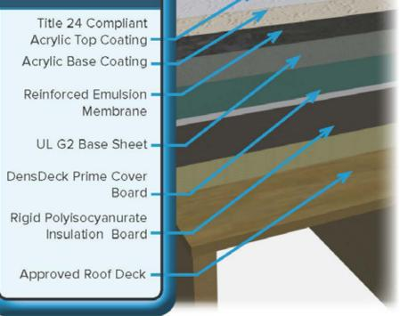
WeatherWeld I-1B-16-30-A is a completely seamless insulated roof system designed for installation over all approved roof deck types, or to recover and enhance existing approved roof systems.
