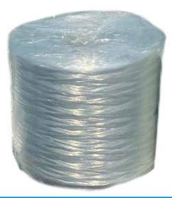
WWFG100 - Fiberglass Roving is continuous filament glass fiber consisting of approximately sixty strands held together loosely in rope form by a special sizing. Roving is designed for spray application using the WeatherWeld 3D Roof Printer to provide reinforcement for WeatherWeld asphalt emulsion coating.
